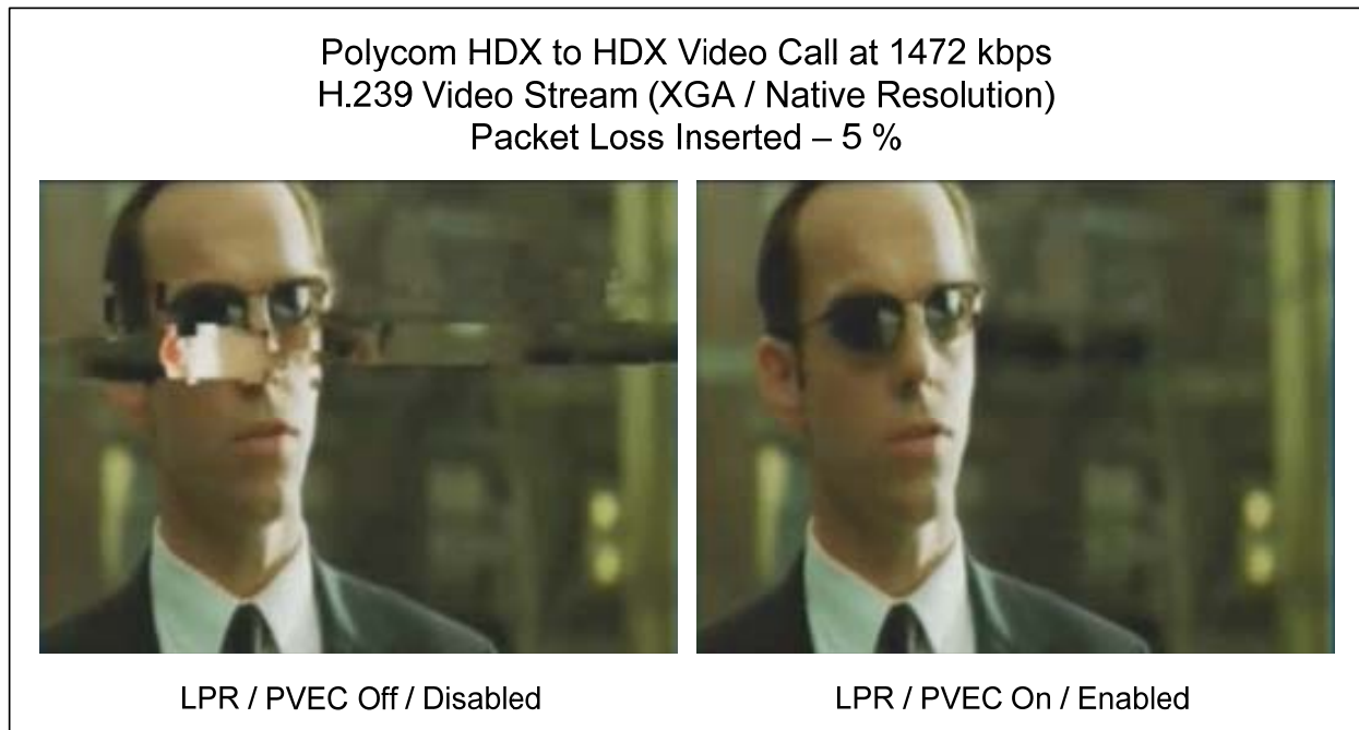
Figure 5: Screenshot of H.239 Test Call w/5% Packet Loss – Without and With LPR
